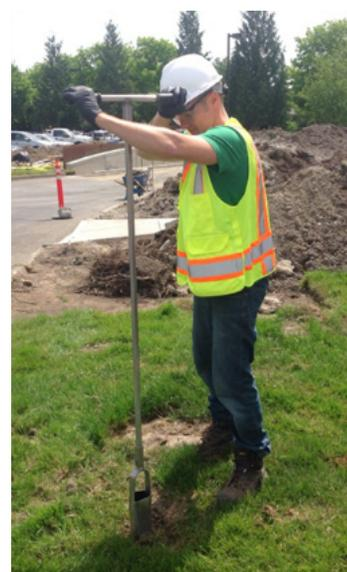
A technician uses a hand auger to dig down into the soil to collect a sample.
